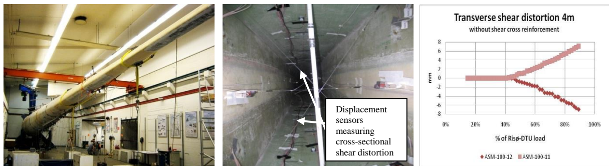
Figure 5 – (a) Full-scale test performed at DTU Wind Energy, showed cross-sectional shear distortion. The blade is loaded at a 30° angle to the flapwise direction, simulating combined flap- and edgewise loads.
