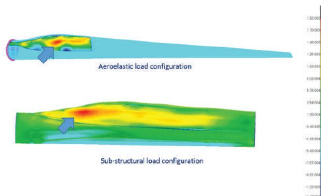
For performance demonstration of the Floor™ technology and the positive effect of the Floor™ solution in the Root-Transition zone, three wind turbine blades have been tested in fatigue with and without the Floor™ technology:
