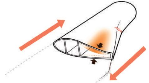
The Root-Transition zone features a complex geometry with tapering panels in different directions. This makes the trailing edge (TE) transition zone vulnerable to out-of-plane deformations especially on medium-sized to large blades.
