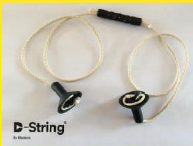
The D-String® technology is made out of three main components: two cones, a fuse and a Vectran Ø2.5 mm string. The solution can be installed up-tower using simple tools from a rigged platform.
