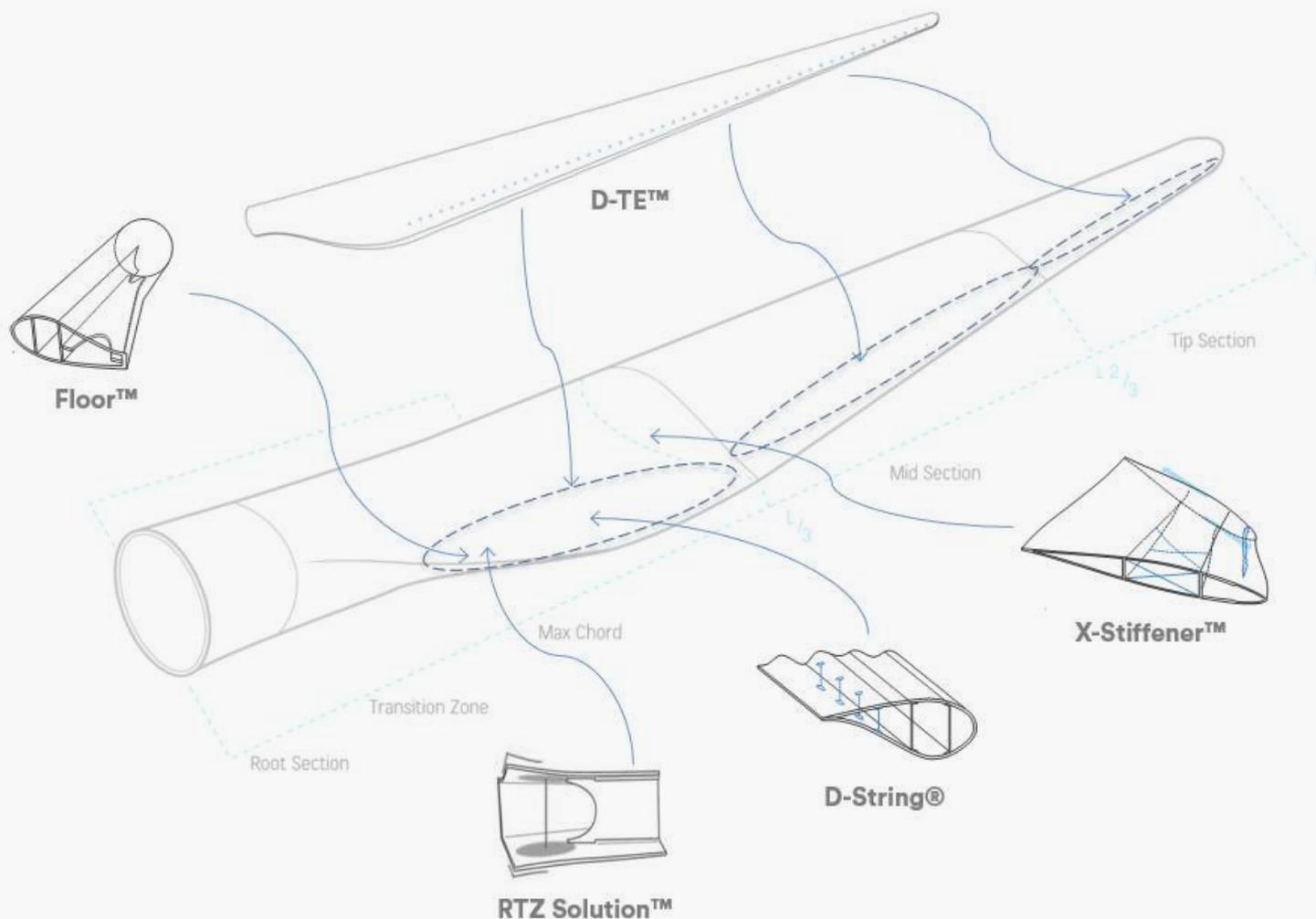
The Bladena retrofit/repair solutions (structural upgrades) are suited to any blade design and solve the specific root cause(s) for the damage(s) to the blade.
