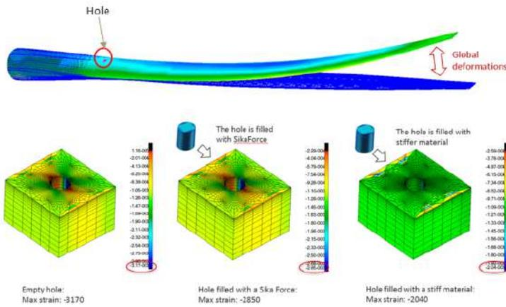
The effect of drilled holes on wind turbine blade panels were investigated and the conclusion of a FE simulation was that the material area around the holes is not reaching the material strength limits.
