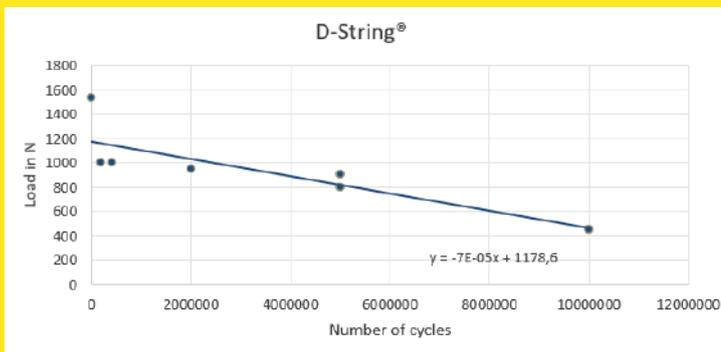
The presented S/N curve shows that the solution can run through 2 million cycles under the pre-determined ultimate loading.
