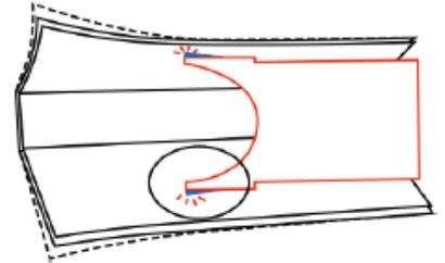
The RTZ Solution™ significantly reduces the peeling stresses in the transition zone area where the aft shear web starts and eliminates defects occurring in the region.
