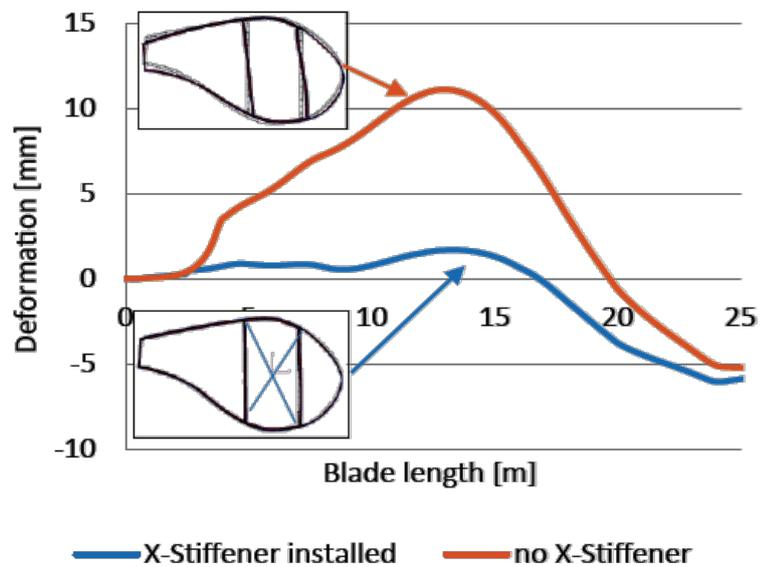
Results from both the test and FEM shows that when a pure torsional moment is applied on a cross-section of a blade, this will develop a cross-sectional shear distortion on a different cross section, in this case towards the root.
