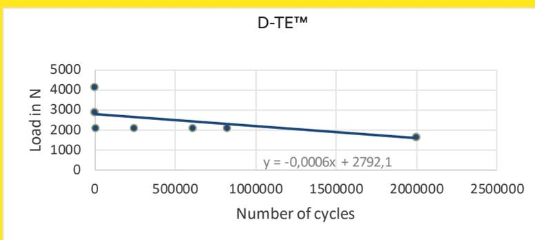
The presented S/N curve shows that the solution can run through 2 million cycles under the pre-determined ultimate loading.
