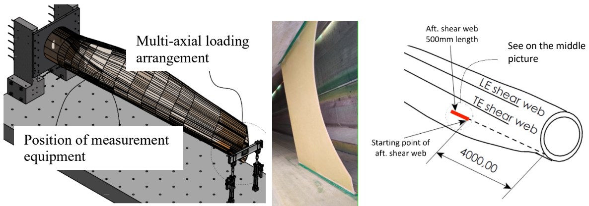
Figure 5. Large-scale strong-floor based test setup, the root section is mounted on a vertical strong-floor and the tip end is mounted onto the load train, the load introduction is explained on Figure 6 (left). Retrofitted aft shear installed in the 2 blade cut-outs (middle). The position of the retrofitted aft shear web illustrated (right).
