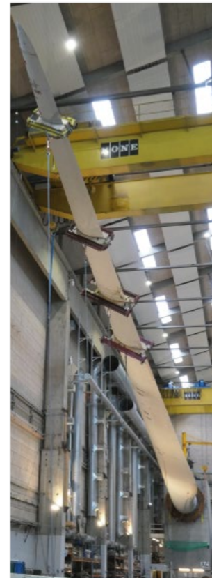
Figure 16: Sketch of a full-scale static test setup with applied torsional load components (left). Photo to the right show a full-scale test of a LM58,7m blade with combined static loads performed at a commercial test center in collaboration with LM-Windpower and Bladena, see ref. [1] EUDP RATZ project.
