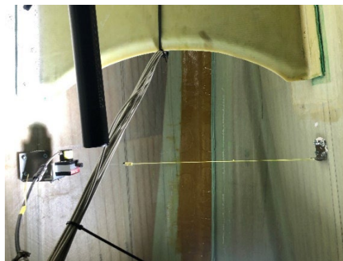
Figure 8. The mounted wire potentiometer measured out-of-plane deformation of the blade panels. The potentiometer was installed 3.8m from the root and 200mm from the retrofitted aft shear web.
