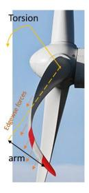
Figure 102: Torsional moment created by the twisting of blade when the blade is subjected to combined loading.
