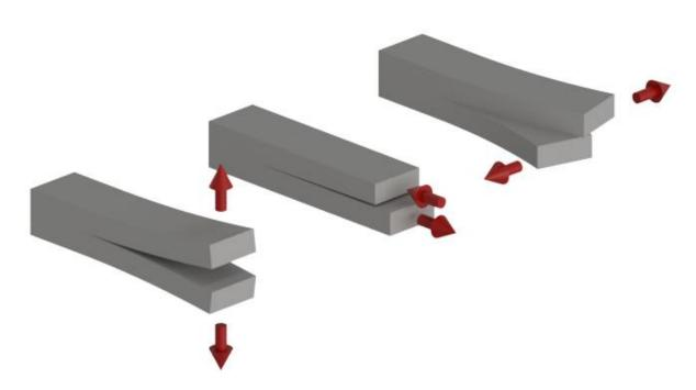
Figure 15 - Modes of crack growth - Mode 1, Mode 2 and Mode 3
