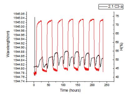
Figure 36 - Fibre response (black line) incorporated in Aerox coatings at position 2 (primer) while varying the humidity (red line) between 45 and 75% relative humidity.
