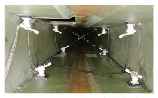
Figure 73 - CSSDS test integration at DTU, installed FCMs inside the blade (left) and test rig (right)
