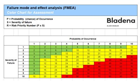
Figure 31 - Failure mode category calculation scheme
