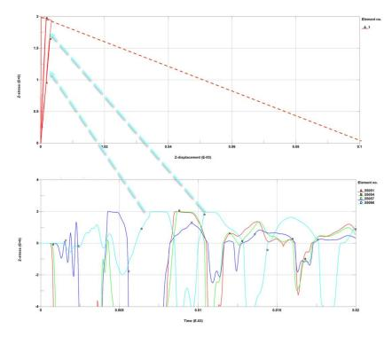
Figure 62 - Stress vs Strain evolution for repeated impacts at interface layer. Cohesive Zone Modelling determined with Peeling testing and its numerical simulation. Ga Adhesive fracture energy loss estimation
