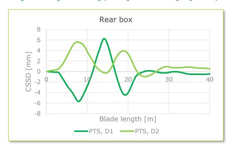
Figure 100: Flapwise loading (Pressure side towards suction side – PTS)
