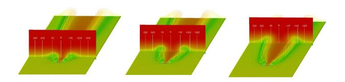
Figure 3 - Flow field in three planes after the vortex generators (planes at 10h-25h & 50h being h the vortex generator height)
