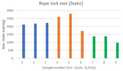
Figure 79 - Column diagram representing the max static load for each test
