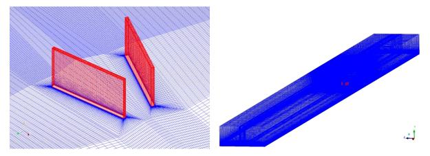
Figure 1- Mesh for the vortex generators pair. 12 million cells.
