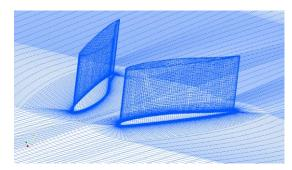
Figure . Vortex generators shapes designed during the ODB project.
