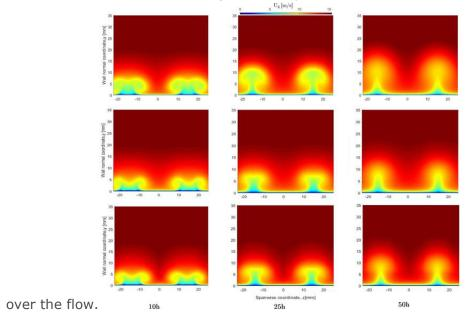
Figure 4 - Velocity fields in three planes right after a vortex generators mounted on a flat plate (10h, 25h and 50h) for three different vortex generator shapes (top rectangular, middle delta and low airfoil shaped)
