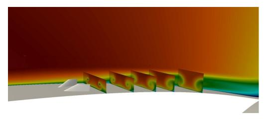
Figure 10 - Vortices after the VGs in the computations from the blade section with LEPS and VGs.
