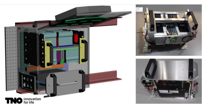
Figure 40 - Hub Cabinet (left), power supply unit sub-assembly (top right) and the interrogator subassembly (bottom right)
