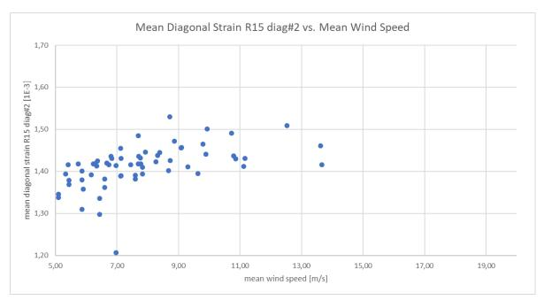
Figure 77 - Measured mean diagonal strain of diagonal #2 at R15 vs. mean wind speed
