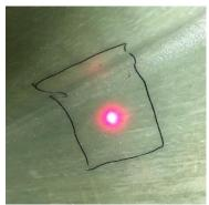
Figure 84 - Photo showing the specially made corner mount insert for laser alignment of brackets
