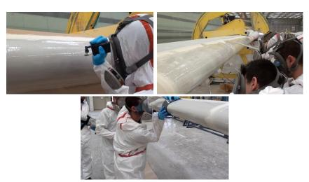
Figure 42 - Application methodologies on wind blades. Left: spray. Centre: roller. Right: filling knife.
