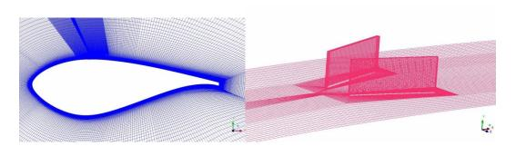
Figure 5 - Mesh used for the computations of the vortex generators mounted in the DU97W300 airfoil.
