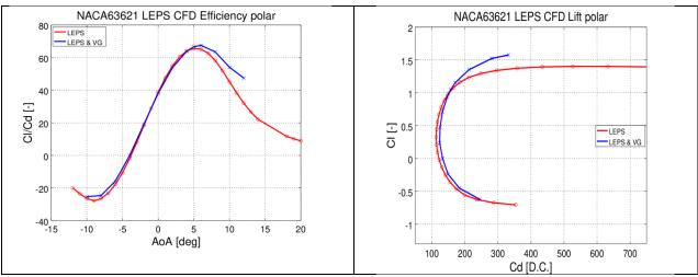
Figure 8 – CFD simulations of the Levenmouth wind turbine section with the leading edge protection system with and without VGs.
