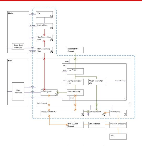
Figure 38 - CSSDS schematic design & interfaces
