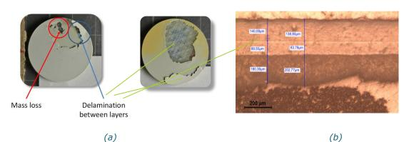
Figure 57 - (a) Rain erosion testing specimens. Erosion failure due to mass loss on surface and interface delamination. (b) Multilayer system microscopy. Two coating layers with different thickness depending on the application method, define an interface that tend to delaminate upon impingement.
