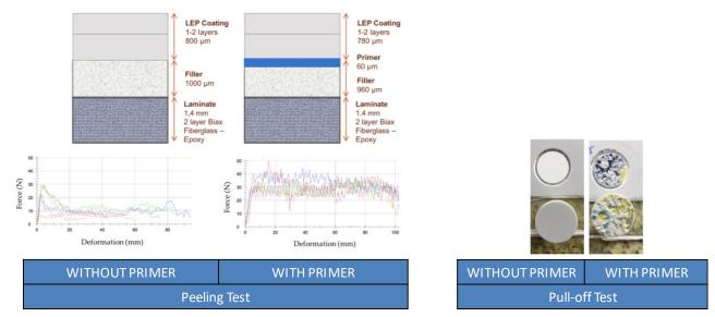
Figure 46 - Pull-off and peeling tests.
