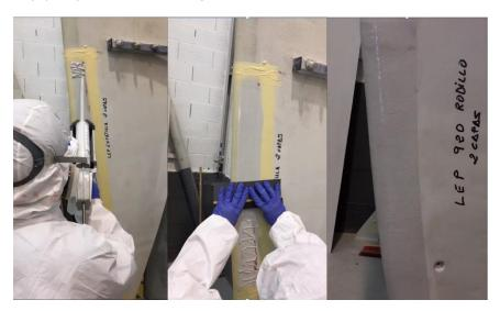
Figure 52 - AHP LEP Service System application (Siemens Gamesa service).
