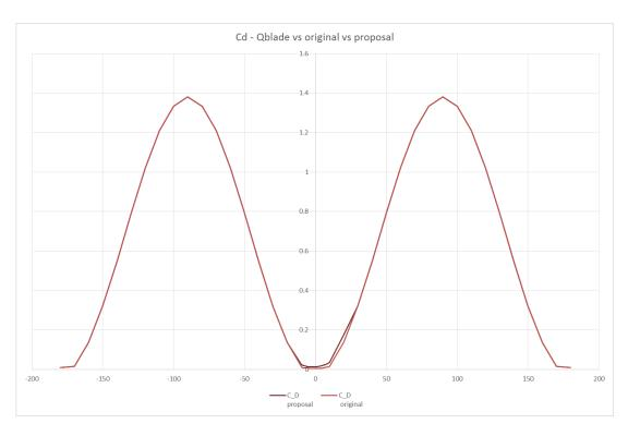
Figure 93 - Plot of drag coefficient for unmodified and modified aerofoils
