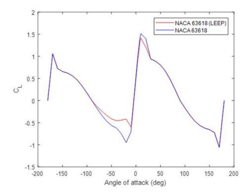
Figure 13 - Plot of lift coefficient for unmodified and modified aerofoils
