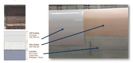
Figure 106. Different layers forming the system wind blade-LEP.
