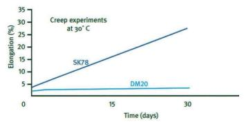
Figure 28 – Creep performance of the rope used for the X-Stiffener™ product
