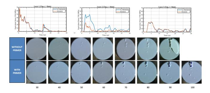
Figure 48 - Simulation of the stresses absorbed with and without primer.
