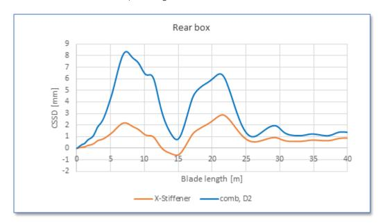
Figure 104: Comparison of cross-sectional shear distortion with and without X-Stiffener. With red with X-Stiffener, with blue without X-Stiffener.
