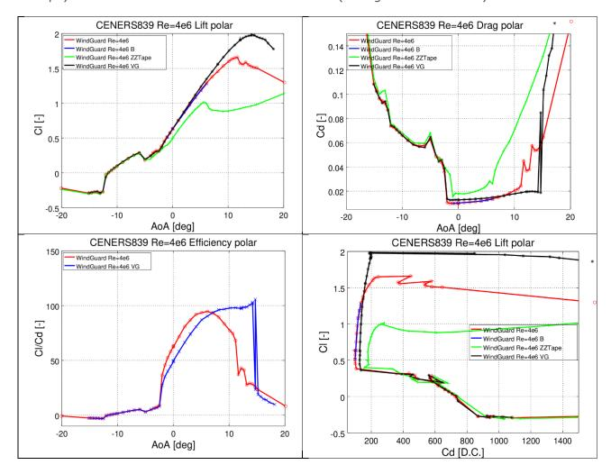
Figure 70 - Measurement of aerodynamic curves of the S839 airfoil in the Windquard wind tunnel.
