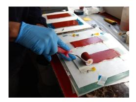
Figure 33 - Incorporation of TNO sensor fibres in Aerox coatings at Aerox laboratories (Valencia, Spain).
