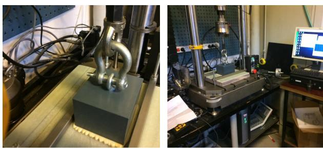
Figure 80 - Test setup: A) interface detail and B) overall setup
