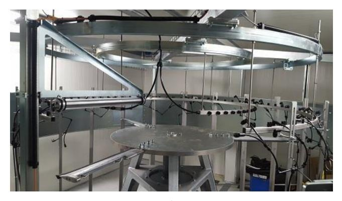
Figure 71 - ORE Catapult Rain Erosion Test Rig
