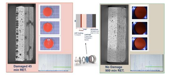
Figure 111. Influence of air bubbles in the RET resistance.
