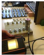
Figure 23 – Adhesion testing for different materials in connection with specified adhesive using SIKA DANMARK facilities in collaboration with DIS & Bladena
