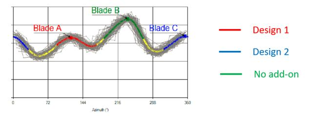
Figure: sound pressure / noise level at different blade position angles at 8.6m/s of wind speed
