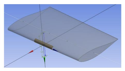
Figure 11 - Parametric FE model of blade/adhesive/tile system
