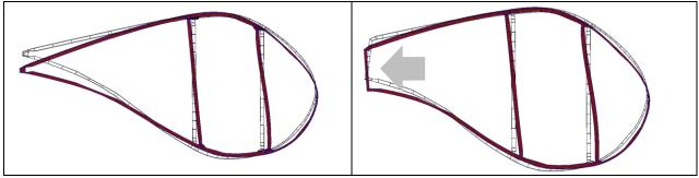
Figure 97: Comparison of a normal sharp trailing edge blade with a modern flatback construction
