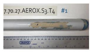
Figure 115. Specimens after 2 hours in RET. Large zone eroded.
