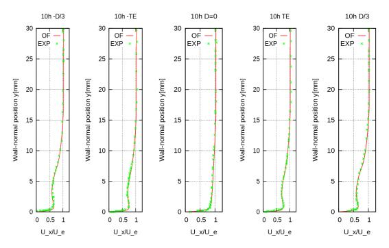
Figure 2 -Velocity profiles in the plane 10h after the vortex generator pair in the middle of the vortex generators, in the trailing edge of each one TE, and in one third of the vortex generator trailing edge separation (0mm, 6.25mm and 10 mm respectively)
