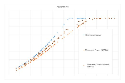
Figure 96 – power curve: ideal vs actual vs estimated performance
