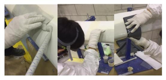
Figure 50 - AHP LEP Service System application (Siemens Gamesa plant)
