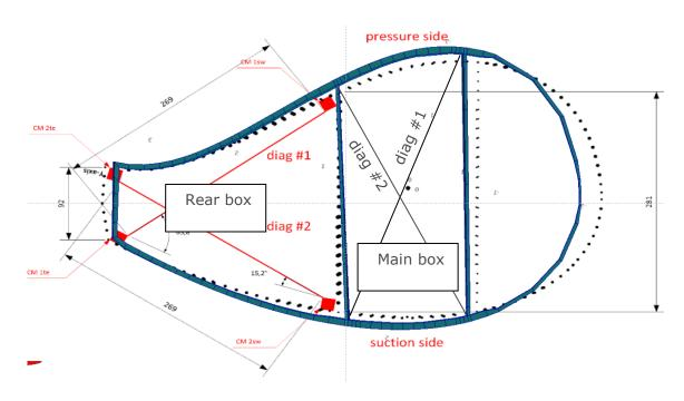
Figure 16: 12m radial position cross section with details on the main and rear boxes
