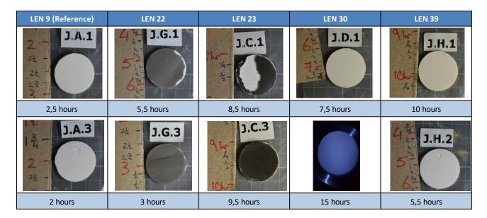
Figure 44 - Results of RETs performed on 5 AHP polymer formulations.
