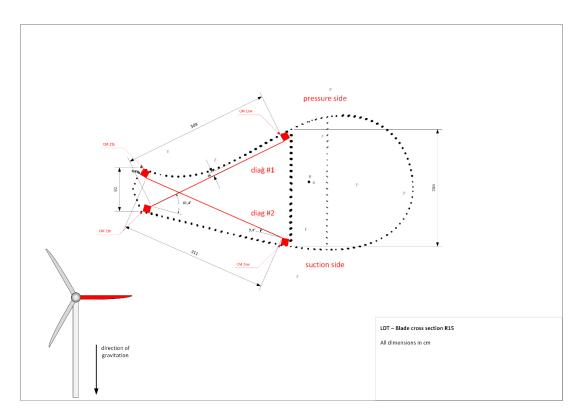
Figure 37 - Cross section R14 of LDT
