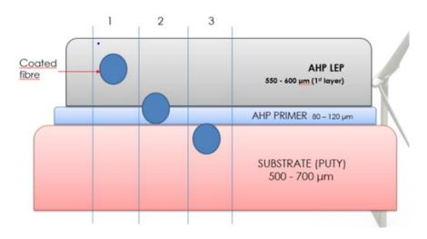
Figure 34 - Fibre positions denoted as 1 (LEP), 2 (primer) and 3 (putty) tested with rain erosion tests (Aerox), mechanical simulations (CEU), humidity (TNO) and rain droplet impact experiments (TNO).
