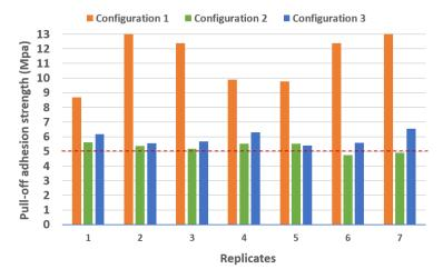
Figure. Pull-off adhesion results for different configurations
