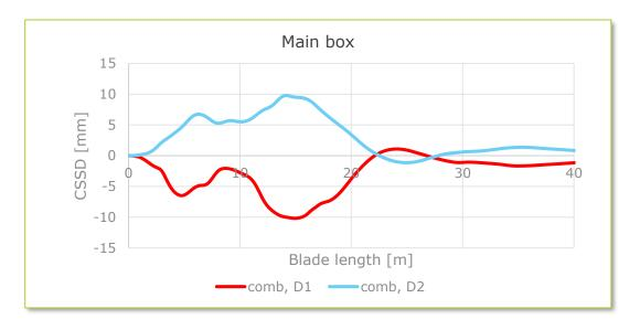
Figure 17: Cross-sectional Shear Distortion in the main box.
