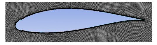
Figure 91 - CFD mesh of blade with 5mm offset on leading edge
