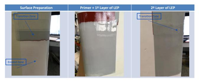
Figure 56 - AEROX AHP LEP repairing procedure.
