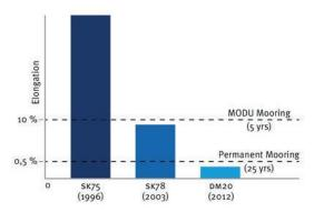
Figure 27 – Elongation performance of the rope used for the X-Stiffener™ product
