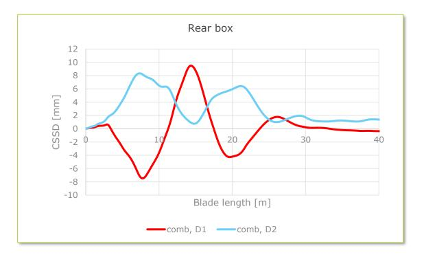
Figure 18: Cross-sectional Shear Distortion in the rear box
