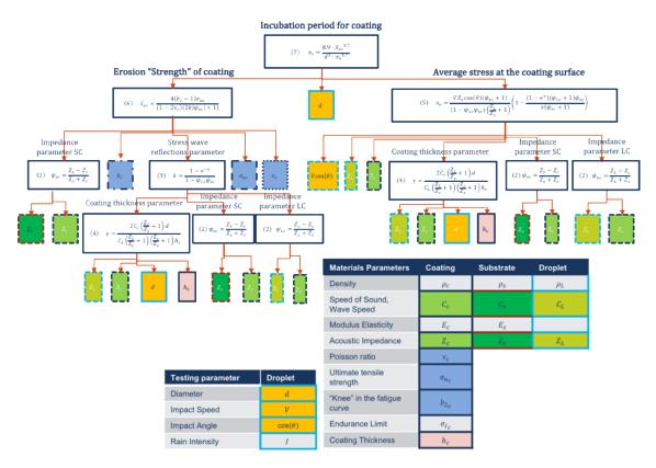
Figure 108. Diagram of material and testing parameters affecting rain erosion performance.
