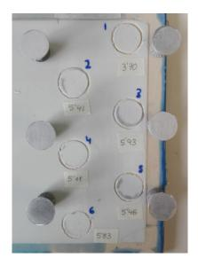
Figure: pull-off adhesion tests done by Siemens Gamesa with Aerox LEP
