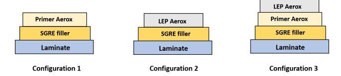
Figure: pull-off configurations tested
