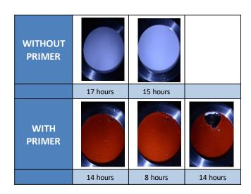
Figure 49 - Evaluation of the influence of the primer on the overall resistance.
