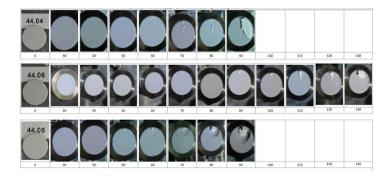
Figure 60 - (a) Rain erosion testing failure evolution due with sanding processing.
