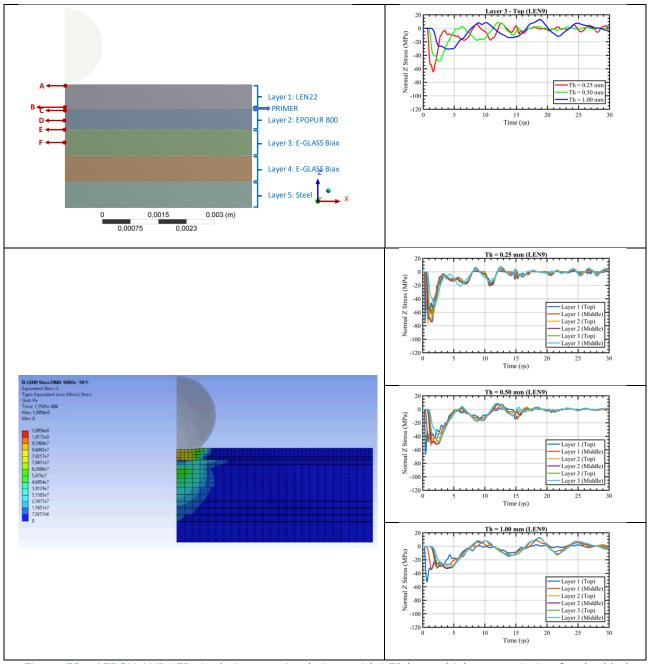
Figure 58 - AEROX AHP LEP single impact simulations with LEP layer thickness variation for the blade multilayer configuration system.
