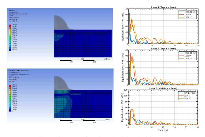
Figure 43 - Simulation of the stress developed through the thickness by different polymers (Epolit GC, LEN9, LEN22. Example of obtained results for tested coupons configurations.
