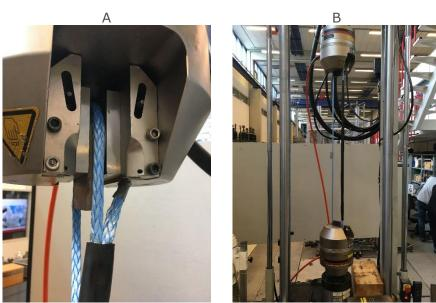
Figure 78 - Test setup: A) boundary conditions and B) overall setup
