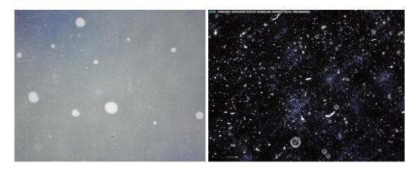
Figure 110. Microscopy images of air bubbles in the LEP.
