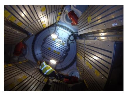
Figure 89 - Technician inspecting cabling inside hub of LDT
