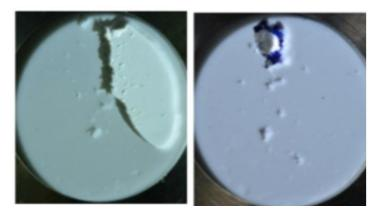
Figure 113. Delamination failure (left) and erosion failure (right).
