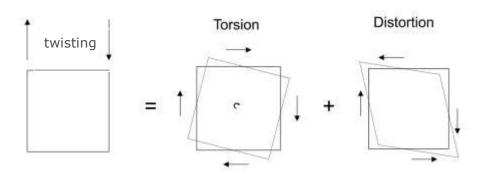
Figure 103: Twisting components: Torsion and Distortion (Cross-sectional shear distortion)
