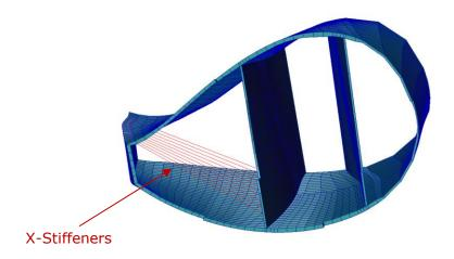
Figure 19: Modelling of X-Stiffeners in the blade
