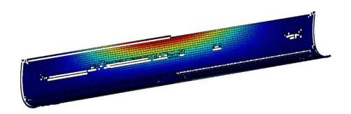
Figure 14 - Plot of Palmgren-Miner damage sum at each point on critical tile
