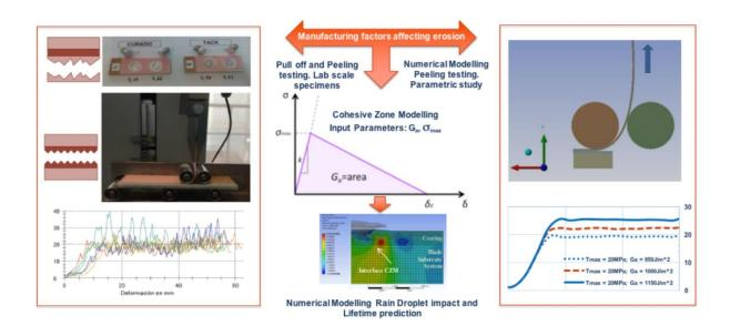
Figure 61 - Proposed methodology for the modelling of manufacturing factors that affect erosion. Input parameters for Cohesive Zone Modelling are determined with Peeling testing and its simulation.
