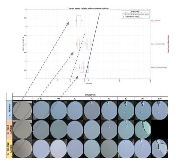
Figure 109. Rain erosion testing analysis for experimental tested (box and whisper plots for wear in red and delamination in blue) and simulated material prototypes. Incubation time for wear failure with primer layer (- -) and without primer (-) on interface.
