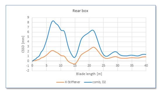
Figure 20: Comparison of cross sectional shear distortion. With red with X-Stiffener; with blue without.
