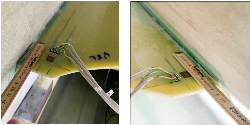
Figure 10. Approximately 10mm crack propagation on the Suction Side (on the left). Approximately 20mm crack propagation on the Pressure Side (on the right).
