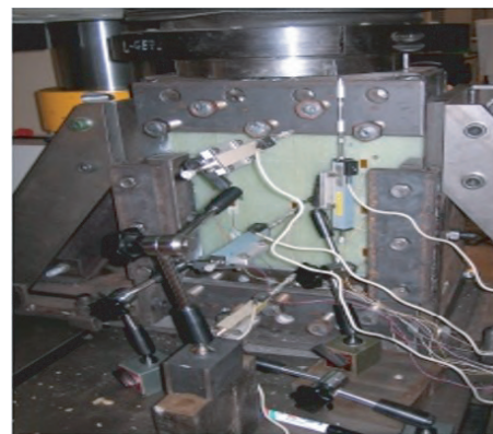
Figure 2 - In-plane compression test demonstrates the over capacity of in-plane strength, shown on Figure 3.
