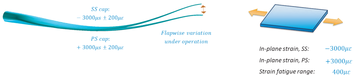
Figure 5 - Longitudinal strain values for a blade exposed to flapwise fatigue test as part of a certification test campaign.
